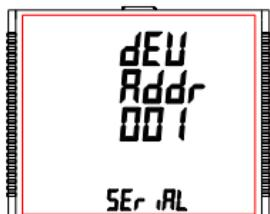
This screen applies to the RS 485 output only. This screen allows the user to set RS 485 address for the meter.
