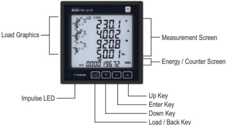
Operation via standard RS485 is also possible. Through this optional interface all the above mentioned parameters can be configured and programmed. For modbus service, it is essential that device address, baud rate and parity should be configured properly.
