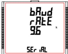
This screen allows the user to set Baud Rate of RS 485 port. The values displayed on screen are in kbaud.
